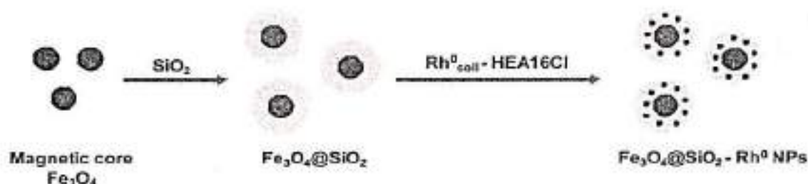
Fig-22: Preparation of Fe_3O_4@SiO_2-Rh^0 NPs
